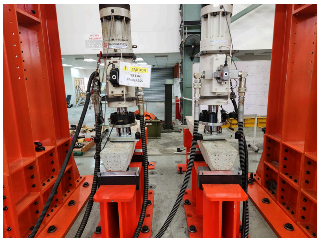
Prestressed railway concrete sleepers testing
